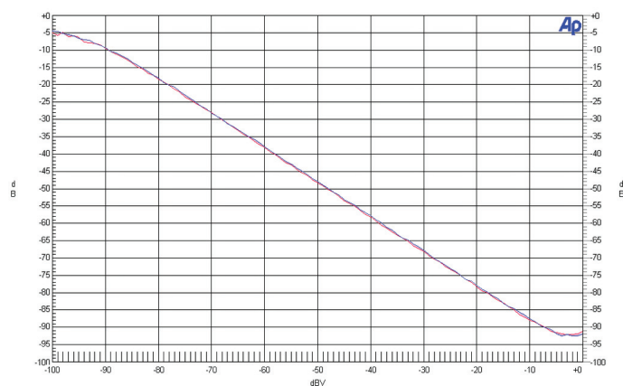
Line Record (path 5) - 10k load THD+N Ratio Versus Input Level
