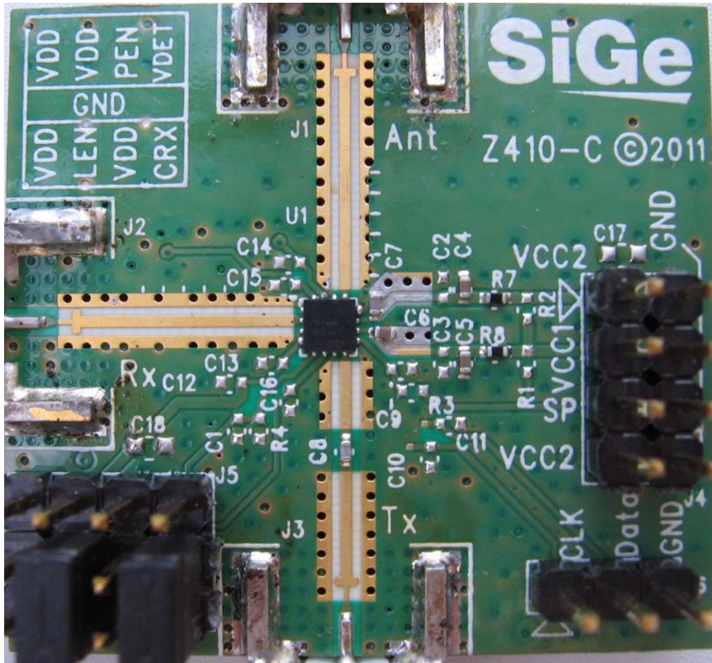
Figure 4. SKY65535-11 Evaluation Board Assembly
