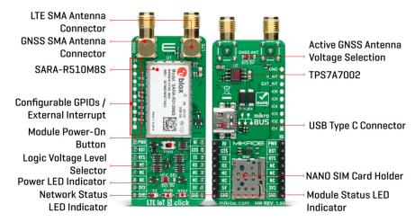
The GNSS RF input of the SARA-R510M8S, designed with  $50\Omega$  characteristic impedance and with an internal DC block, is suitable for both active and/or passive GNSS antennas due to the built-in SAW filter followed by an LNA in front of the integrated high performing u-Blox M8 concurrent positioning engine.
