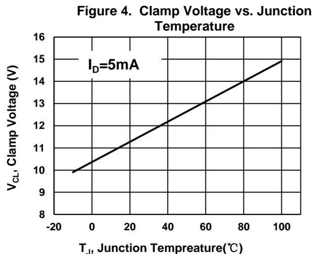
Figure 4. Clamp Voltage vs. Junction Temperature
