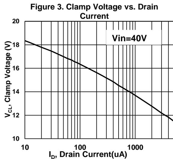
Figure 3. Clamp Voltage vs. Drain Current
