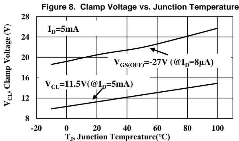
As shown in Figure 8, in the practical application of DMZ1015E/DMX1015E, with the increase of device temperature, its output voltage will also increase, and the drain-source voltage will decrease, so that the device's power consumption will also decrease. In this way, the temperature of DMZ1015E/DMX1015E will decrease. This negative feedback mechanism enables DMZ1015E/DMX1015E to reach a stable thermal equilibrium state.
