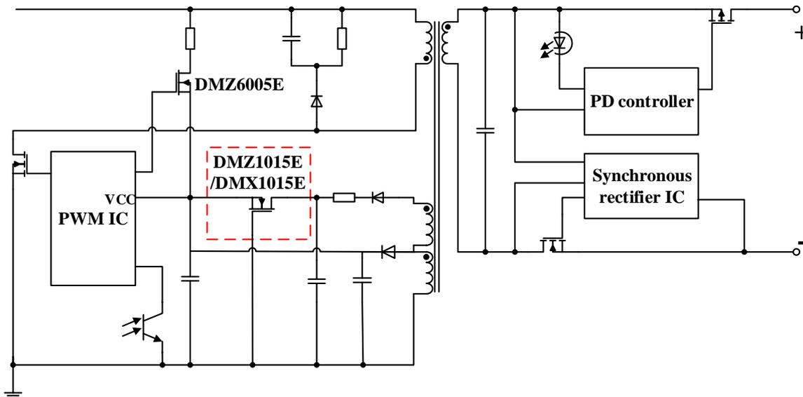
**Figure 6. Circuit with DMZ1015E/DMX1015E**
