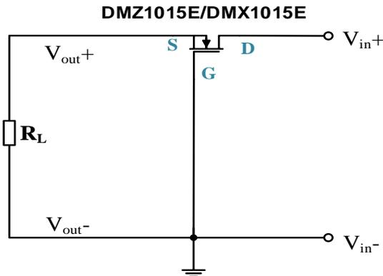
Figure1. Drain Current  $I_D$  is decided by Load Resistance
