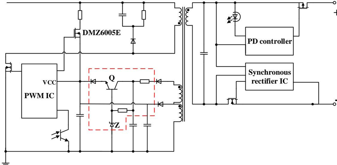
**Figure 5. Normal Circuit with Transistor and Diode**
