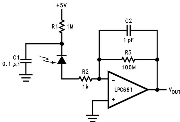
**Note:** A 5V bias on the photodiode can cut its capacitance by a factor of 2 or 3, leading to improved response and lower noise. However, this bias on the photodiode will cause photodiode leakage (also known as its dark current).
