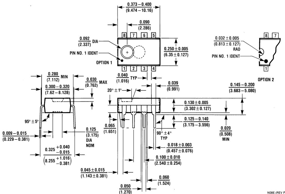
**8-Pin Molded Dual-In-Line Package (N)**
