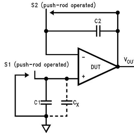
**FIGURE 10. Simple Input Bias Current Test Circuit**
