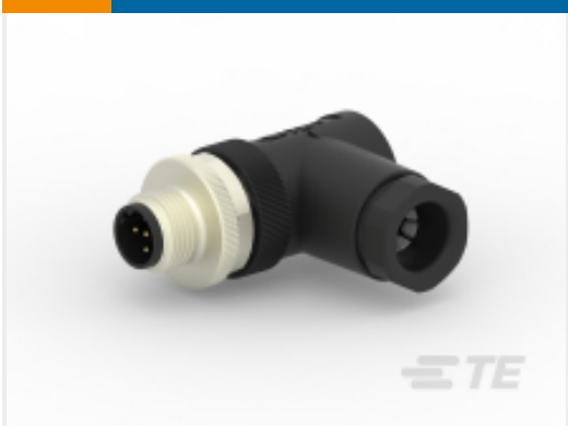
TE Part #T4113402051-000 M12,MALE,RA,B CODE,5P,PG9,GOLD
