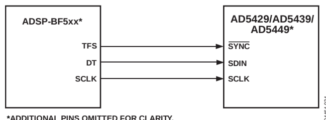
Figure 51. ADSP-BF5xx SPORT-to-AD5429/AD5439/AD5449 Interface
