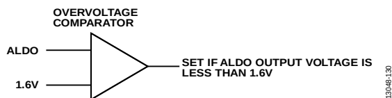
Figure 123. Analog LDO Monitor
