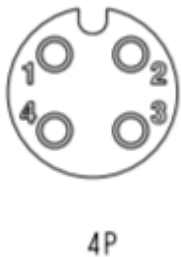
Front view of connector Pin 1: (+), Pin 2 (-), Pins 3 & 4: N/C
