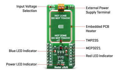
Heater Click allows PCB temperature adjusting and monitoring as it have embedded trace resistor on top layer of PCB. Resistor is made from copper 1oz thick and a pattern of 0.1mm wide track 1950mm long, this give us about 10 ohm resistance at 25 degrees Celsius.
