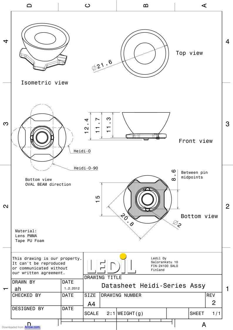
Luminaire: Ledil Oy CA12435\_HEIDI-ON-90 (Cree XP-G 71Im @ 250mA) Efficiency=88% Lamps: 1 x Cree XP-G 71Im @ 250mA
