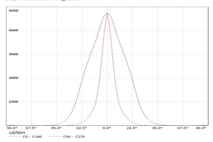
Luminaire: Ledil Oy CA12434\_Heidi-ON (Cree XP-G 71Im @ 250mA) Efficiency=88% Lamps: 1 x Cree XP-G 71Im @ 250mA
