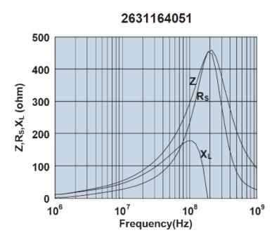
Impedance, reactance, and resistance vs. frequency.
