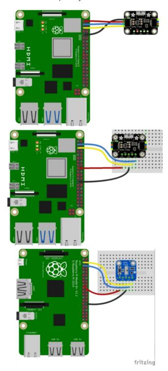
Pi 3V3 to sensor VIN (red wire on STEMMA QT version) Pi GND to sensor GND (black wire on STEMMA QT version) Pi SCL to sensor SCL (yellow wire on STEMMA QT version) Pi SDA to sensor SDA (blue wire on STEMMA QT version)
