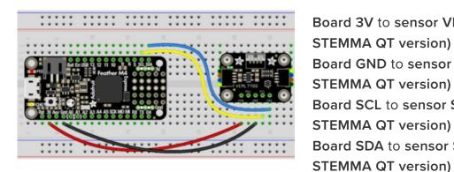
Board 3V to sensor VIN (red wire on STEMMA QT version) Board GND to sensor GND (black wire on STEMMA QT version) Board SCL to sensor SCL (yellow wire on STEMMA QT version) Board SDA to sensor SDA (blue wire on
