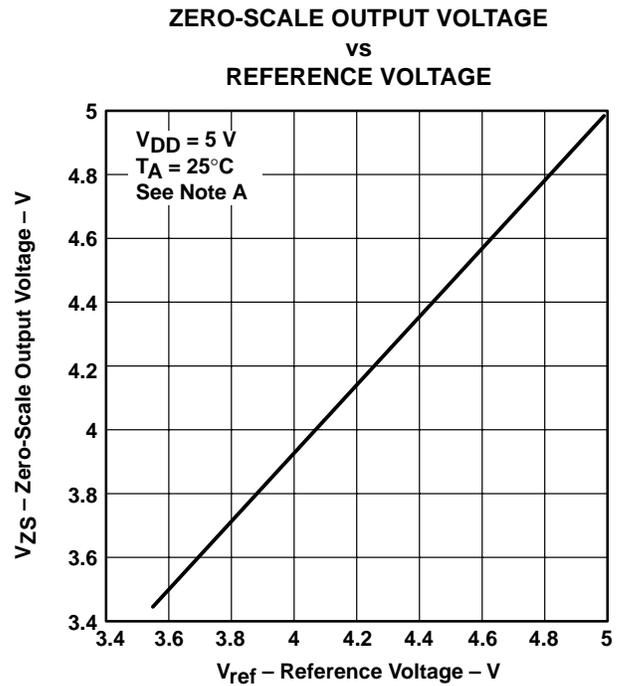
NOTE A:  $V_{ref}$  is relative to ANLG GND.  $V_{DD}$  is the voltage between ANLG  $V_{DD}$  and DGTL  $V_{DD}$  tied together and ANLG GND and DGTL GND tied together.
