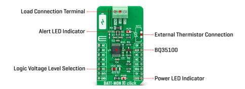
This device measures the BT input using the integrated delta-sigma ADC, scaled by the internal translation network, through the ADC. A calibration process determines the translation gain function. It can also operate in three distinct modes: accumulator (ACC), state-of-health (SOH), and end-of-service (EOS) mode. The device can be configured and used for only one of these modes in the field, as it is not intended to be able to switch between modes when in regular use.
