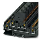
Fuse modular terminal block, fuse type: Glass / ceramics / ..., fuse type: G / 5 x 20, nom. voltage: 500 V, nominal current: 28 A, connection method: Push-in connection, 1 level, Rated cross section: 4 mm<sup>2</sup>, cross section: 0.2 mm<sup>2</sup>- 6 mm<sup>2</sup>, connection method: Push-in connection, 2nd level, Rated cross section: 4 mm<sup>2</sup>, cross section: 0.2 mm<sup>2</sup>- 6 mm<sup>2</sup>, mounting type: NS 35/7,5, NS 35/15, color: black
