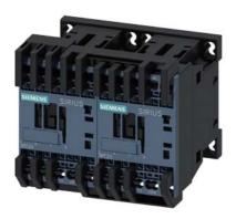
reversing contactor assembly, AC-3e/AC-3, 7 A, 3 kW / 400 V, 3-pole, 230 V AC, 50/60 Hz, spring-loaded terminal, electrical and mechanical interlock
