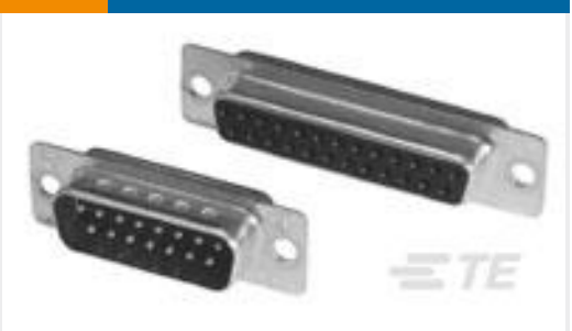
TE Part #5-747909-2 15 Rcpt Solder Cup, Gold Flash
