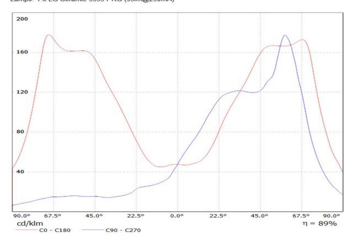
Luminaire: LEDiL Oy CA12787\_STRADA-K\_(LG3535) Eff. 96,1% Lamps: 1 x LG Ceramic 3535 PKG (95Im@250mA)
