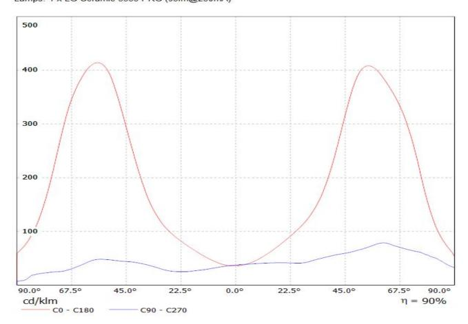
Luminaire: LEDiL Oy 2FA11992\_STRADA-T-DN-EP\_(LG3535) Eff. 89,1% Lamps: 1 x LG Ceramic 3535 PKG (95lm@250mA)
