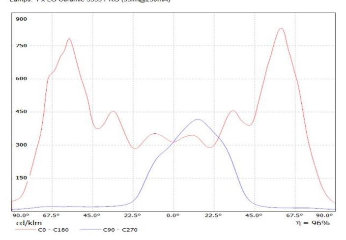
Luminaire: LEDiL Oy CA11416\_STRADA-T-DN\_(LG3535) Eff. 89,1% Lamps: 1 x LG Ceramic 3535 PKG (95lm@250mA)
