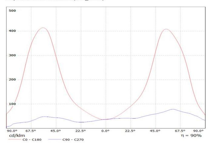
Luminaire: LEDiL CA12050\_STRADA-FT\_(LG3535) Eff. 86% Lamps: 1 x LG Ceramic 3535 PKG (95lm@250mA)
