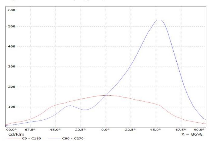
Luminaire: LEDiL Oy CA12087\_STRADA-FW\_(LG3535) Eff. 88,2% Lamps: 1 x LG Ceramic 3535 PKG (95Im@250mA)
