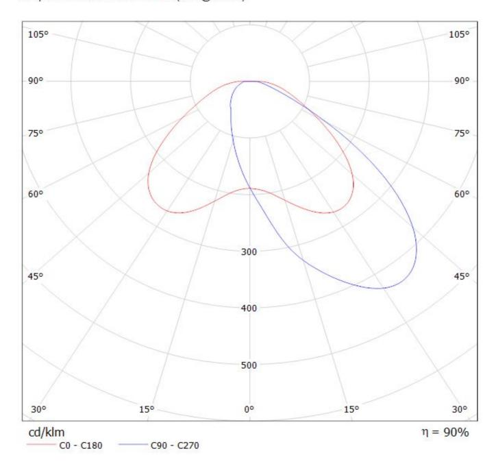
Luminaire: LEDiL Oy 2FA11993\_STRADA-T-DW-EP\_(LG3535) Eff. 90,4% Lamps: 1 x LG Ceramic 3535 PKG (95Im@250mA)
