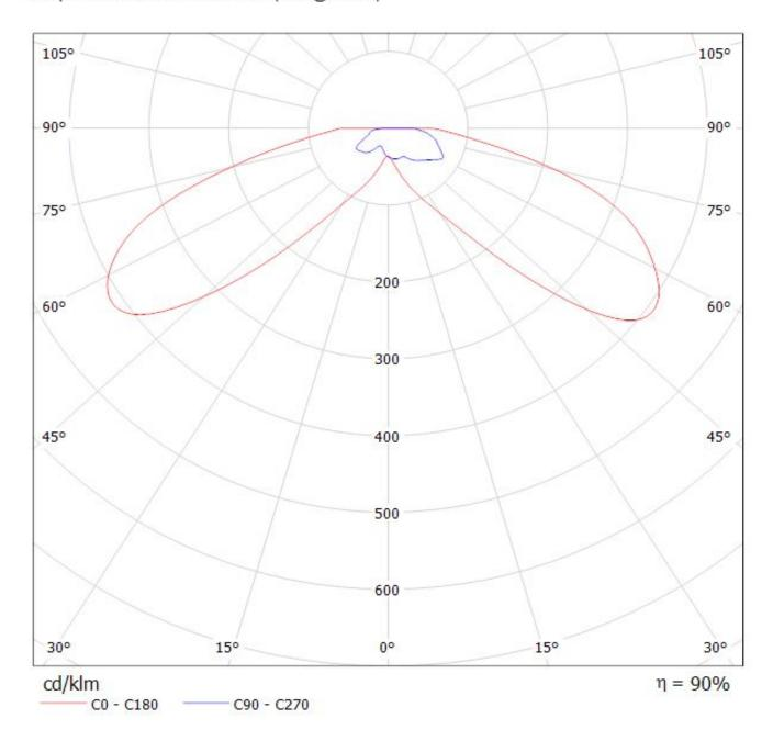
Luminaire: LEDiL CA12050\_STRADA-FT\_(LG3535) Eff. 86% Lamps: 1 x LG Ceramic 3535 PKG (95Im@250mA)
