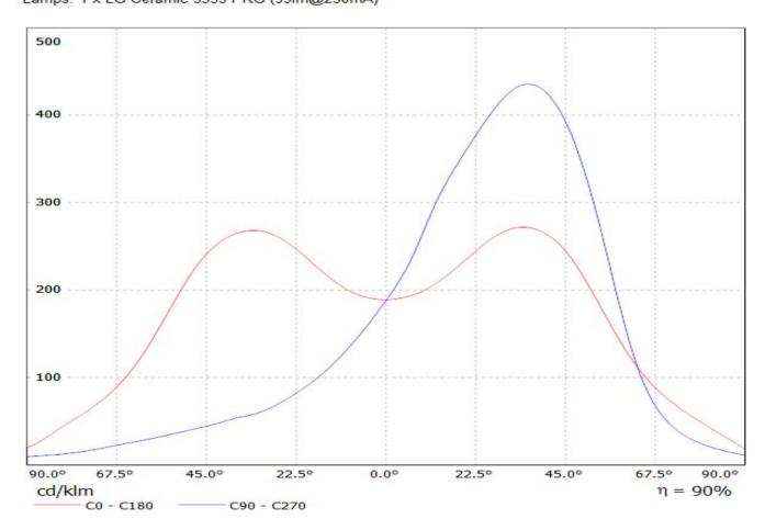
Luminaire: LEDiL Oy 2FA11993\_STRADA-T-DW-EP\_(LG3535) Eff. 90,4% Lamps: 1 x LG Ceramic 3535 PKG (95lm@250mA)
