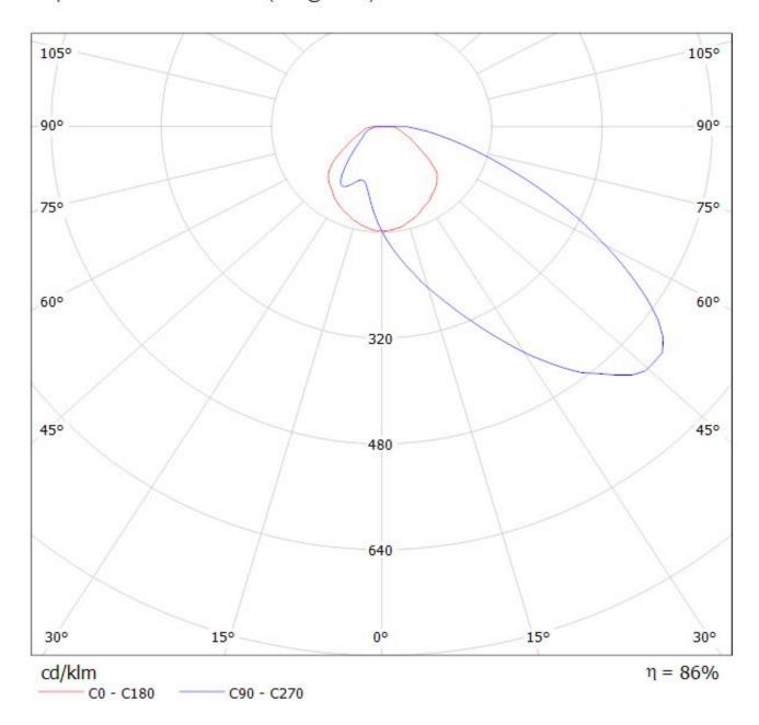
Luminaire: LEDiL Oy CA12087\_STRADA-FW\_(LG3535) Eff. 88,2% Lamps: 1 x LG Ceramic 3535 PKG (95lm@250mA)
