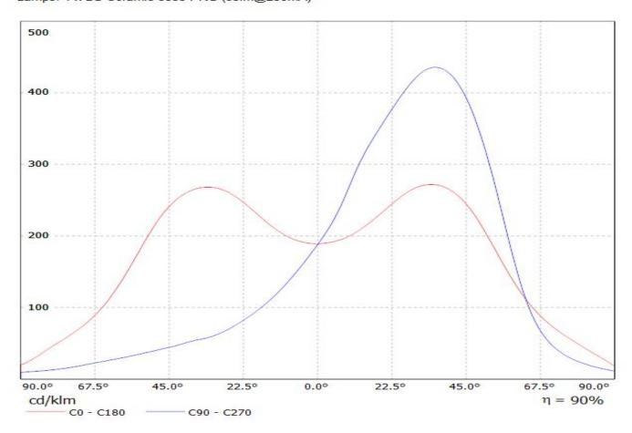
Luminaire: LEDiL Oy CA11426\_STRADA-T-DW\_(LG3535) Eff. 90,4% Lamps: 1 x LG Ceramic 3535 PKG (95lm@250mA)
