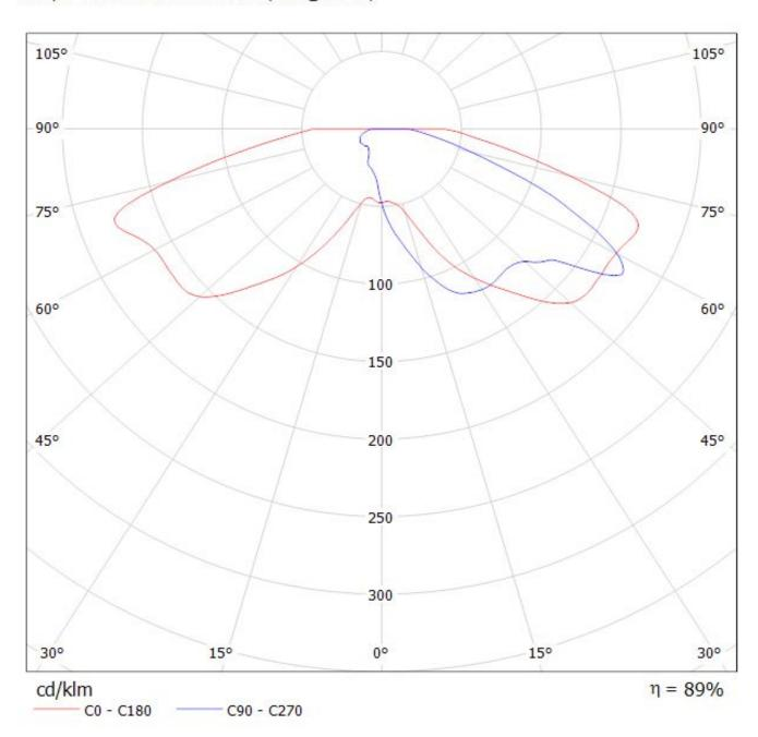
Luminaire: LEDiL Oy CA12787\_STRADA-K\_(LG3535) Eff. 96,1% Lamps: 1 x LG Ceramic 3535 PKG (95lm@250mA)
