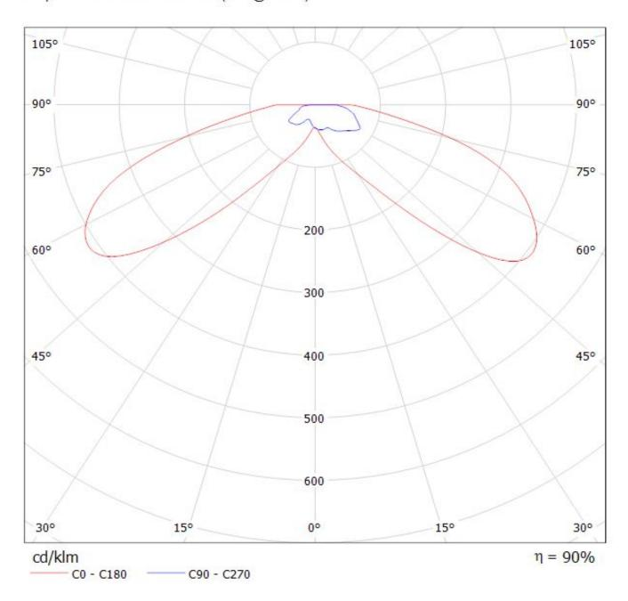
Luminaire: LEDiL Oy 2FA11992\_STRADA-T-DN-EP\_(LG3535) Eff. 89,1% Lamps: 1 x LG Ceramic 3535 PKG (95lm@250mA)
