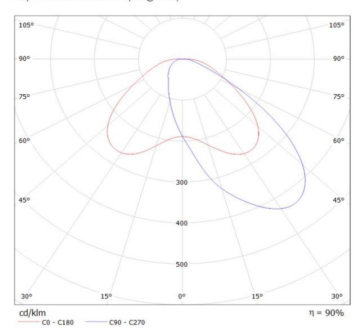
Luminaire: LEDiL Oy CA11426\_STRADA-T-DW\_(LG3535) Eff. 90,4% Lamps: 1 x LG Ceramic 3535 PKG (95Im@250mA)
