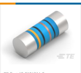
TE Part #2-2176316-2 MELF SMA\_A 5K6 0.1% 15PPM 0207 1W
