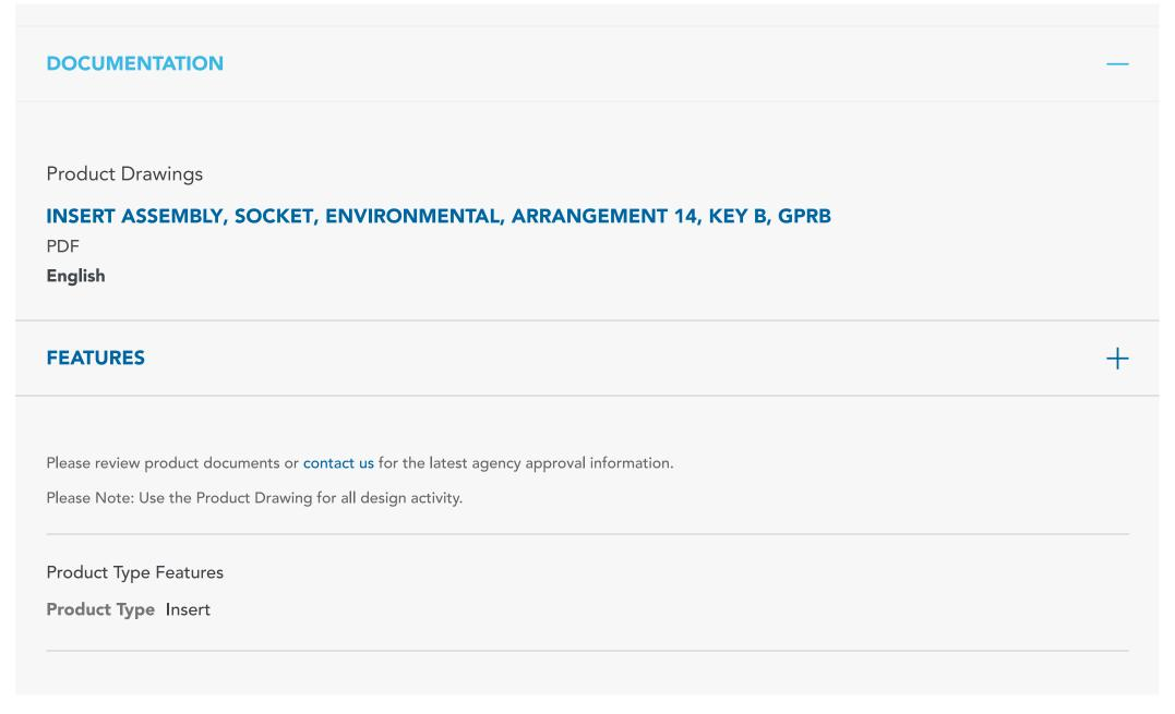
**Configuration Features Number of Positions 14** Keying B **Body Features Insert Type** Environmental Insert Style Socket Interfacial Seal With Module Material Thermoplastic, Thermoset Rear Grommet With **Contact Features** Contact Type Socket Number of Poles 14 **Dimensions** Wire Range (AWG) 14, 15 Operation/Application For Use With GPRB **PRODUCT COMPLIANCE** Statement of Compliance **Statement of Compliance** PDF
