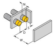
All non-flush mountable *uprox*\*+ threaded barrel sensors can be screwed in up to the top edge of the barrel. In this mounting position, the sensor operates safely with a 20 % reduced switching distance.
