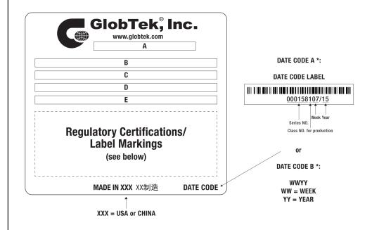
A=Medical/ICT/ITE/Household use Power Supply B=P/N: (料号) TR9CH9440LCPIMR6B C=Model (型号) GTM961800P17018-T3 D=Input (输入)100-240V~, 50-60Hz, 2.2A E=Output (输出)18.0 V == 9.44 A, 170.00W
