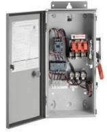
Slim Line Pump Control Panel NEMA size 1 Three phase full voltage Solid-state overload relay OLR amp range 5.5-22A 110/120V 50/60Hz Coil 30A fusible disconnect 30A/250V fuse clip 1NC / 1NO auxiliary contacts HOA Sel. Sw. <(>&<)> Start/Stop 3-point power terminal block 3-point control terminal block 3-point ground lug Enclosure NEMA type 3/3R Weather proof outdoor use
