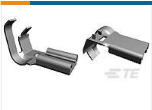
TE Part #41802 250 FASTON FLAG REC 18-12 AWG TPBR
