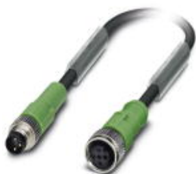
Sensor/actuator cable, 3-position, PUR halogen-free, black-gray RAL 7021, Plug straight M8, on Socket straight M12, A-coded, cable length: 4 m
