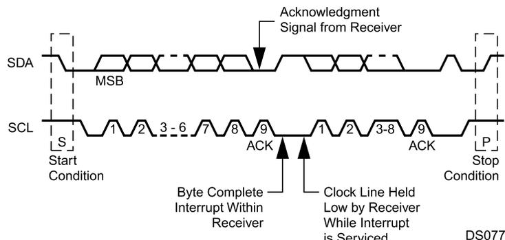
Figure 24-3. ACCESS.bus Data Transaction
