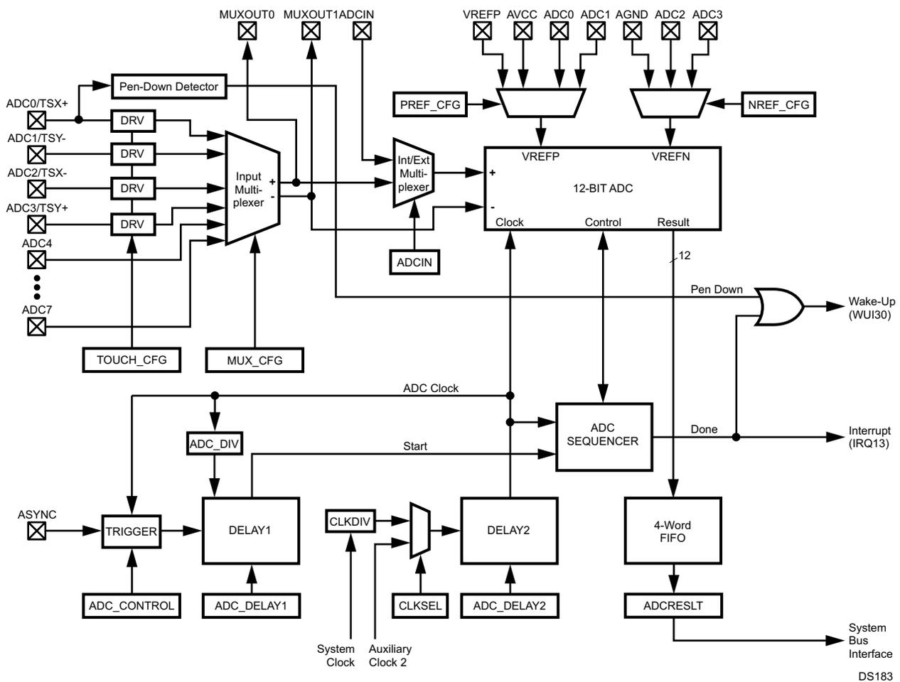
Figure 16-1. Analog to Digital Converter Block Diagram
