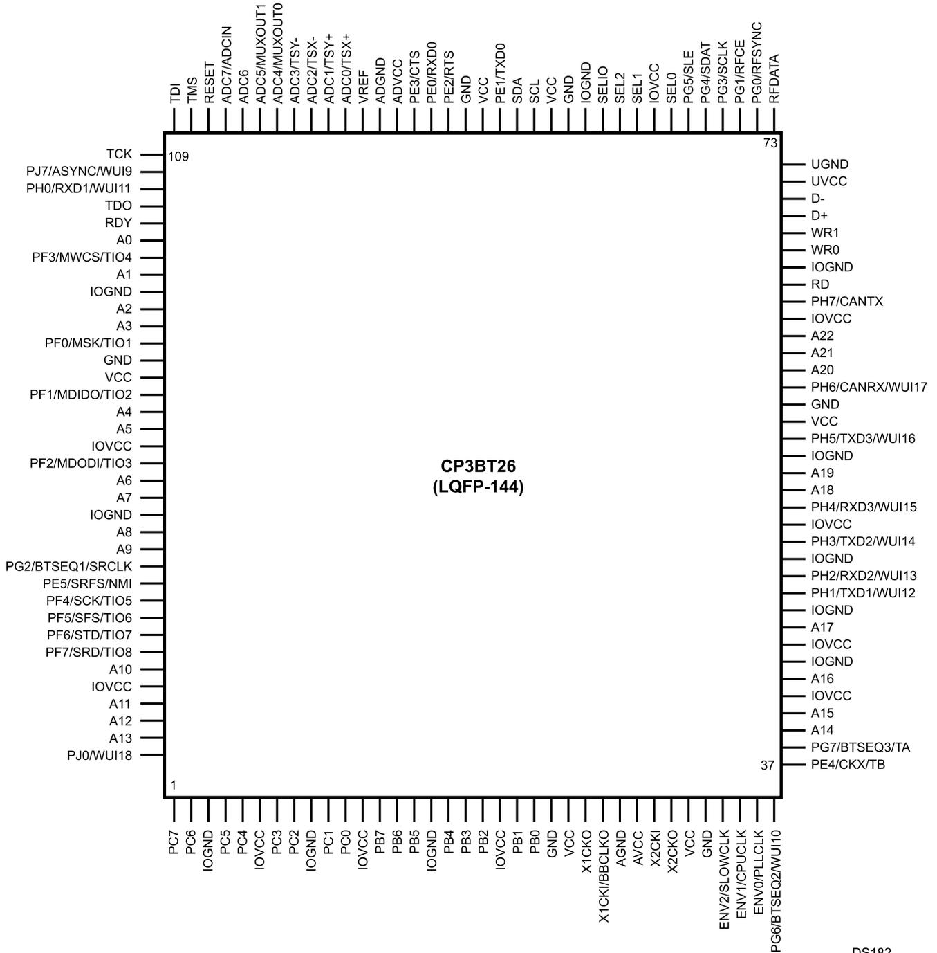
Figure 31-2. CP3BT26 in the LQFP-144 Package (Top View)
