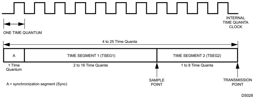
**Figure 19-11. Bit Timing**
