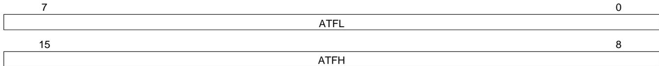
**ATFL** The Audio Transmit Low Byte field represents the lower byte of the transmit FIFO location currently addressed by the Transmit FIFO Write Pointer (TWP).
