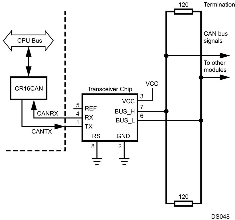
Figure 19-31. External Transceiver
