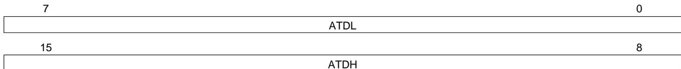
**ATDL** The Audio Transmit DMA Low Byte field holds the lower byte of the audio data.
