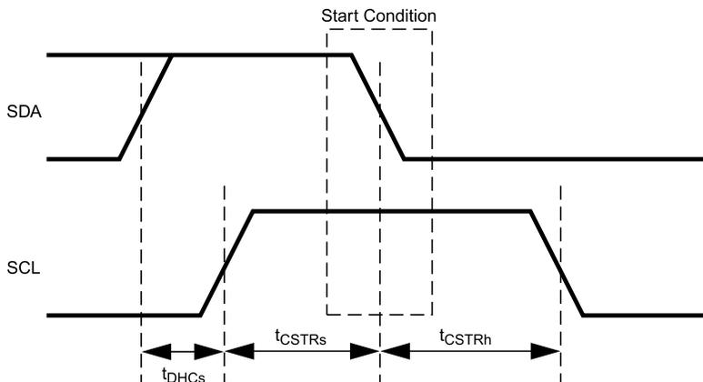
Note: In the timing tables the parameter name is added with an "o" for output signal timing and "i" for input signal timing.
