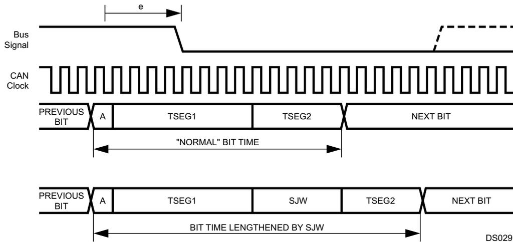
Figure 19-12. Resynchronization ( $e > SJW$ )
