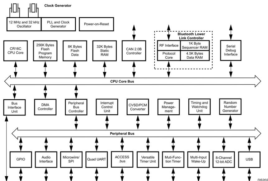
Figure 1-1. Block Diagram
