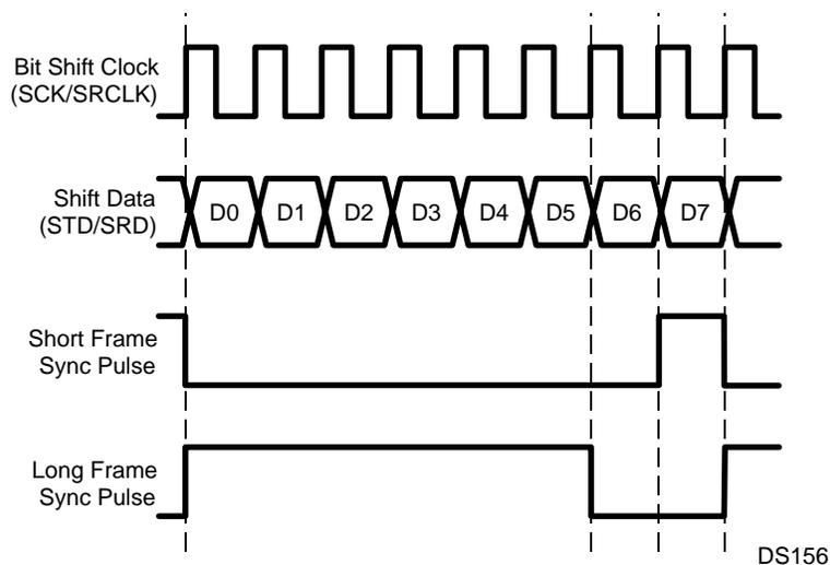
**Figure 20-7. Short and Long Frame Sync Pulses**
