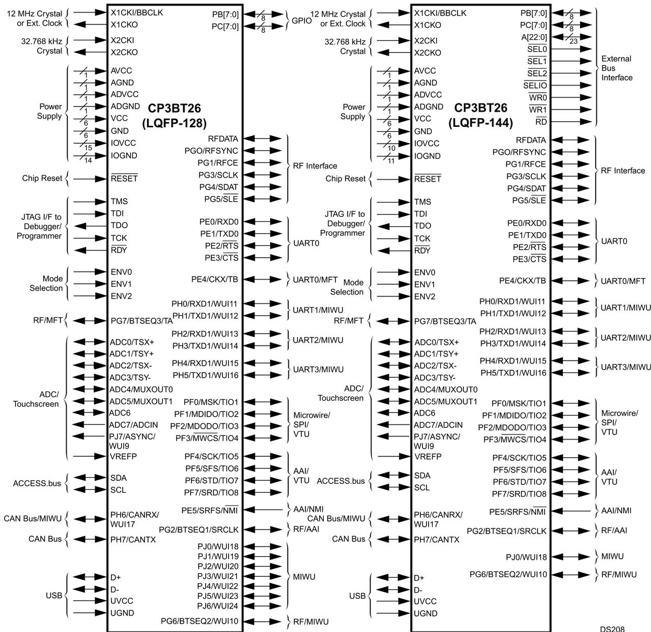
(1) Some pins may be enabled as general-purpose I/O-port pins or as alternate functions associated with specific peripherals or interfaces. These pins may be individually configured as port pins, even when the associated peripheral or interface is enabled. [Table 4-1](#) describes the device signals for the LQFP-128 package. [Table 4-2](#) describes the device signals for the LQFP-144 package.
