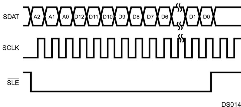
Figure 15-5. Serial Interface 16-bit Fast-Write Timing
