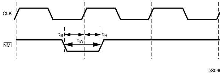
Figure 30-2.  $\overline{\text{NMI}}$  Signal Timing
