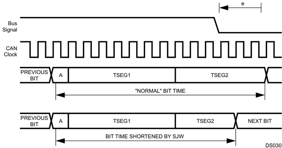
Figure 19-13. Resynchronization ( $e < -SJW$ )
