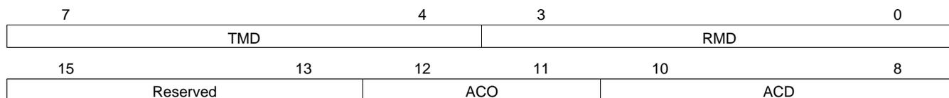
**RMD** The Receive Master DMA field specify which slots (audio channels) are supported by DMA, that is, when a DMA request is asserted to the DMA controller. If the RMDn bit is set for an assigned slot n (RXDSA<sub>n</sub> = 1), a DMA request n is asserted, when the ARDRn is full. If the RXDSA<sub>n</sub> bit for a slot is clear, the RMDn bit is ignored. The following table shows the receive DMA request scheme.
