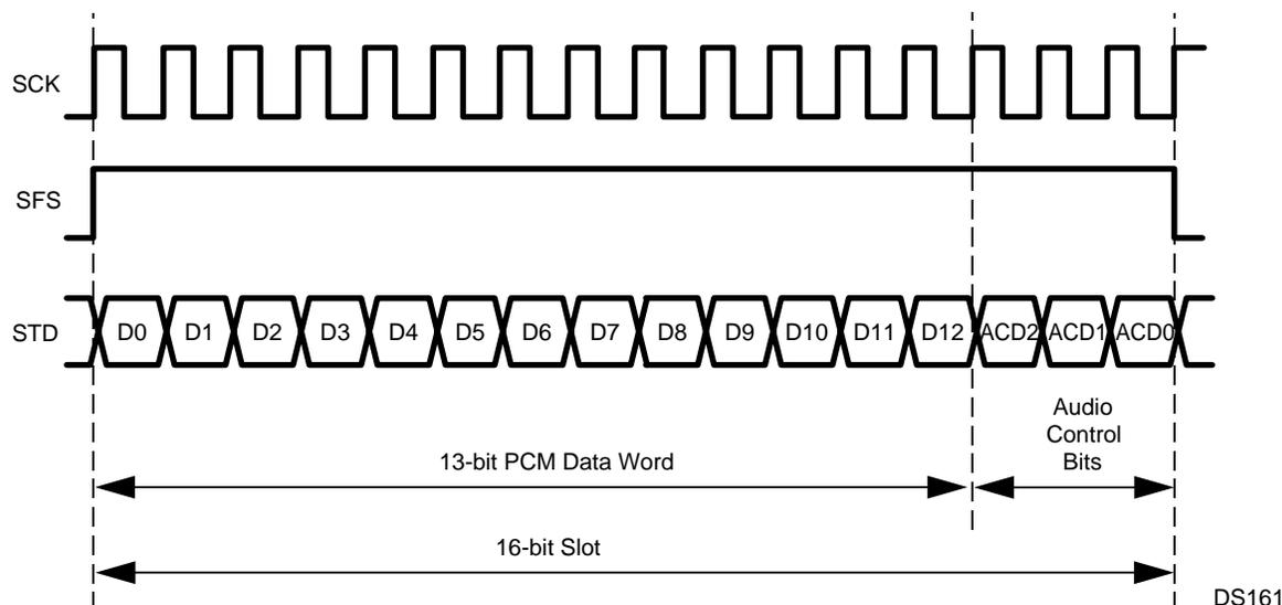
Figure 20-8. Audio Slot with Audio Control Data
