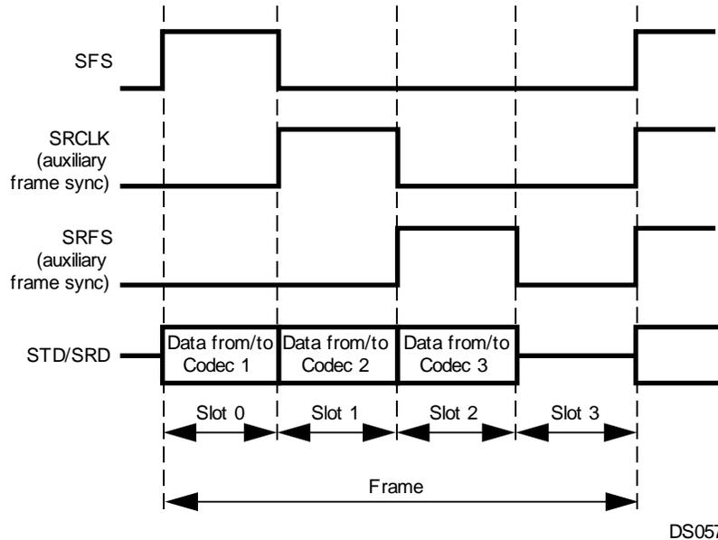
**Figure 20-5. Accessing Three Devices in Network Mode**
