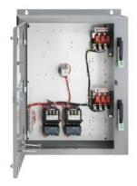
Duplex starter w/ alternator, Size 3, Three phase full voltage, Solid-state overload relay, OLRelay amp range 25-100A, 110V 50HZ / 120V 60HZ coil, Combination type, Two 100A disconnect switches, Encl NEMA type 4X 304 S-steel Water/dust tight noncorrosive
