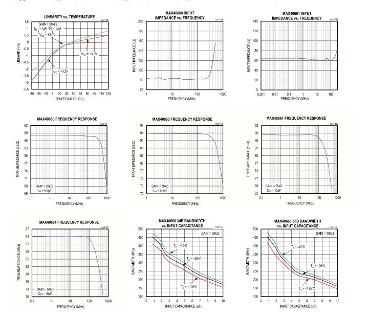
$(V_{CC} = +3.3V, C_{IN} = 0.5pF (MAX40660), C_{IN} = 8pF (MAX40661), T_A = +25°C; unless otherwise noted.)$
