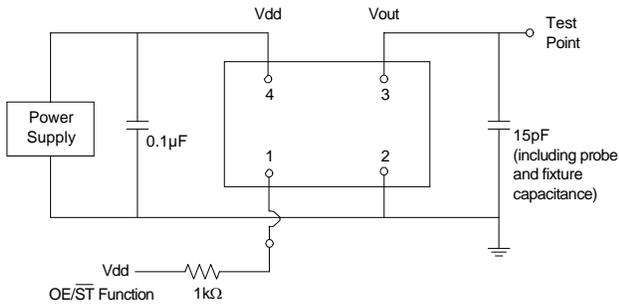
**Figure 2. Test Circuit**
