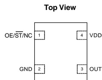
Figure 1. Pin Assignments
