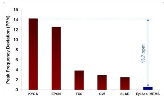
Figure 4. Power Supply Noise Rejection<sup>[4]</sup>
