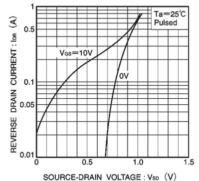
Fig.9 Reverse drain current vs. source-drain voltage ( II )
