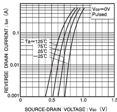
Fig.8 Reverse drain current vs. source-drain voltage ( I )
