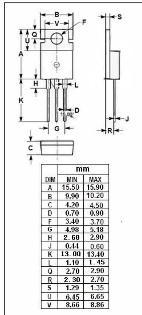
**isc N-Channel MOSFET Transistor****FQP10N20C****ELECTRICAL CHARACTERISTICS****T<sub>c</sub>=25°C unless otherwise specified**
