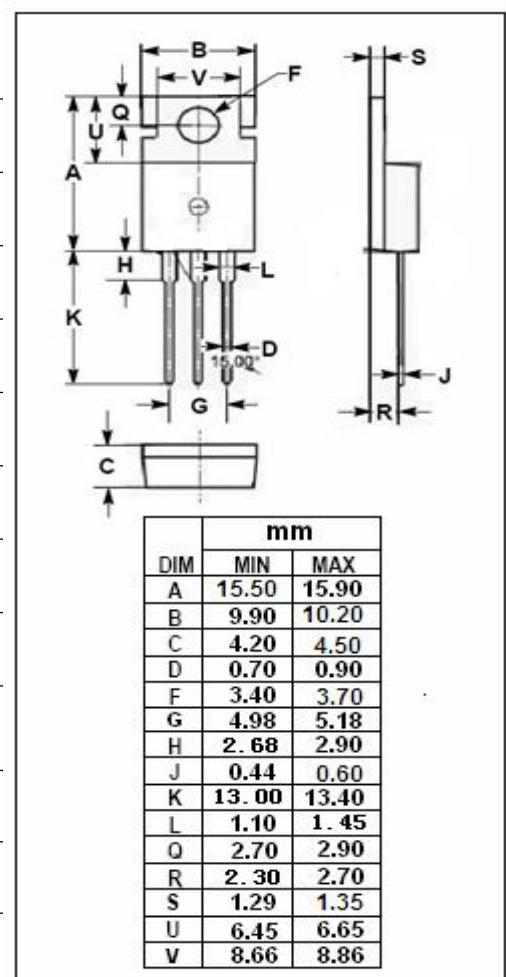
**isc N-Channel MOSFET Transistor****IPP052N06L3,IIPP052N06L3****ELECTRICAL CHARACTERISTICS****T<sub>c</sub>=25°C unless otherwise specified**
