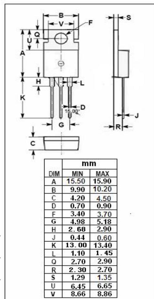
**isc N-Channel MOSFET Transistor IRFB38N20D, IIRFB38N20D****ELECTRICAL CHARACTERISTICS****T<sub>c</sub>=25°C unless otherwise specified**
