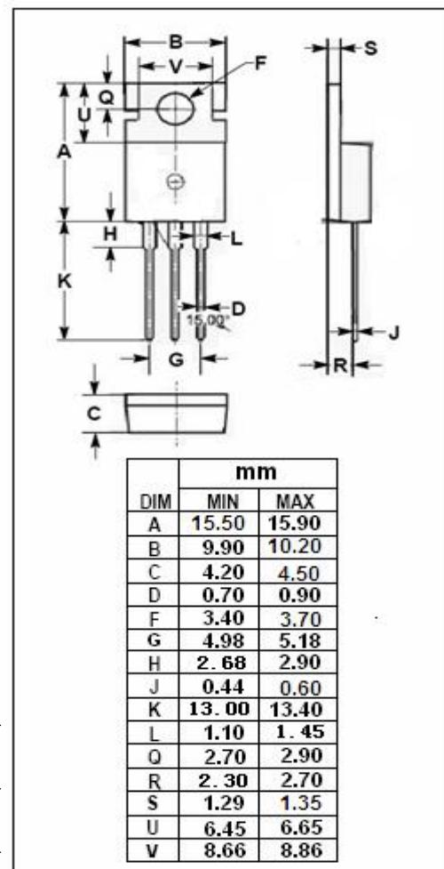
**isc N-Channel MOSFET Transistor****SPP21N50C3, ISPP21N50C3****ELECTRICAL CHARACTERISTICS****T<sub>c</sub>=25°C unless otherwise specified**
