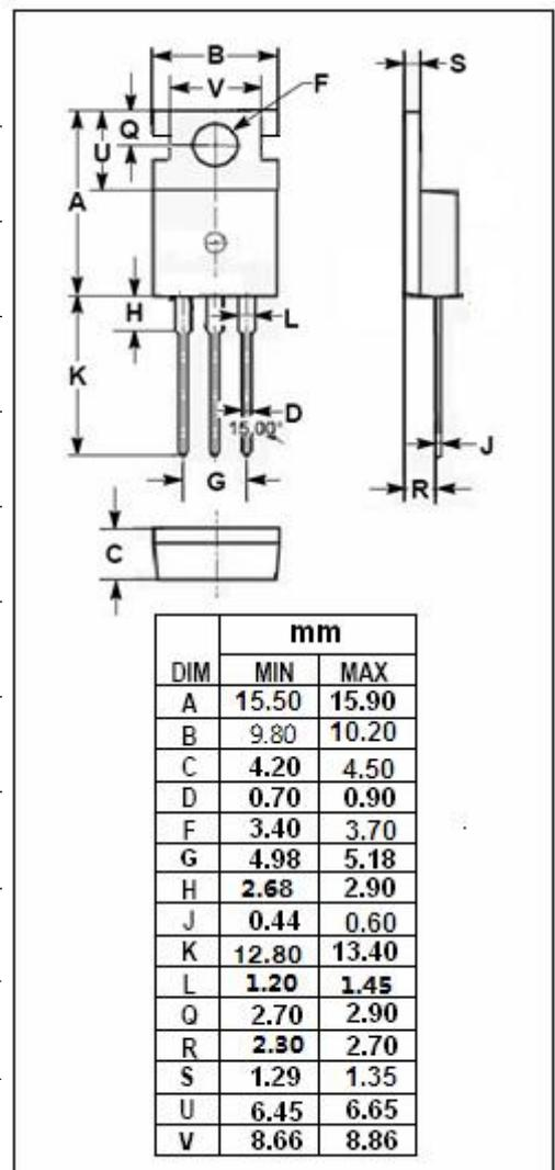
**Isc N-Channel MOSFET Transistor****TK56E12N1****ELECTRICAL CHARACTERISTICS**T<sub>c</sub>=25°C unless otherwise specified
