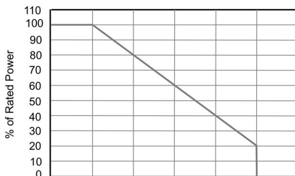
Fig3. Power Derating Curve
