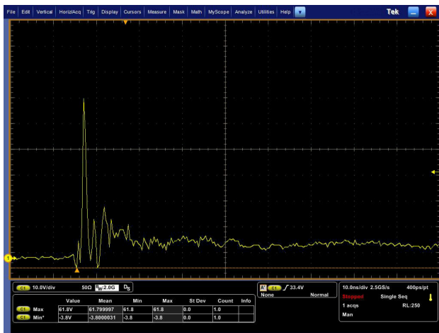
Figure 3. ESD Clamping Voltage Screenshot Positive 8 kV Contact per IEC61000-4-2
